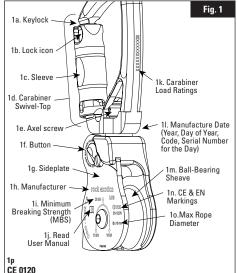
EN 362:2004/B, EN 12278:2007, EN 12275:2013/B Locking Carabiner, Type B (Base), Type H (For Munter Hitch Belay), Type K (Via Ferrata) Notified body controlling the manufacturing of this PPE: SGS United Kingdom Ltd. (CE 0120), 2028 Worle Parkway, Wes-
